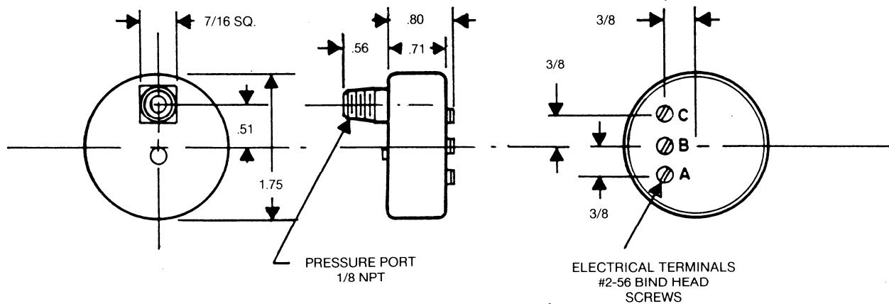
*Designed as a low cost pressure transducer, Model 9000 utilizes a ni-span C bourdon tube sensing element usually found in more expensive units. Lower cost is achieved via standardization of pressure ranges, available resistances and linearity ranges. Unit provides infinite resolution through use of conductive film resistance element. Typical applications include pressure monitoring in process control, agriculture, automotive testing and refinery operations.*
