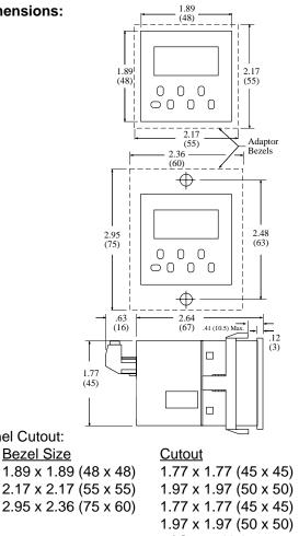
w/ Screw Holes Adaptor bezels supplied: 2.17 x 2.17 (55 x 55) or 2.95 x 2.36 (75 x 60)
